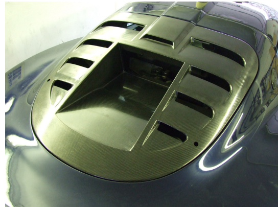
Unpainted tailgate awaiting slats & Dzus fasteners
